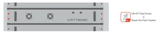
**Step3.** Install the battery module from bottom to top, and install the Sub-Master BMS in the top of the cabinet, use M6×10 screws and break the paint gasket to secure the Sub-Master BMS to the cabinet.
