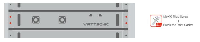
**Step3.** Install the battery module from bottom to top, and install the Sub-Master BMS in the top of the cabinet, use M6×10 screws and break the paint gasket to secure the Sub-Master BMS to the cabinet.
